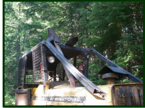
FIGURE 1. Shovel mounted on the top of a skidder.
