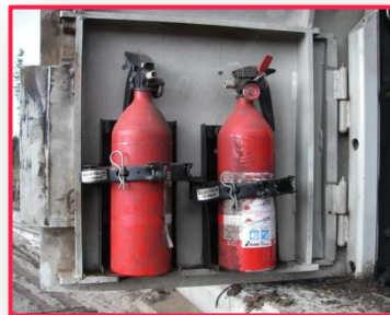
FIGURE 13. Fire extinguishers mounted on an excavator.
