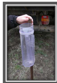
FIGURE 6. A rain gauge.
