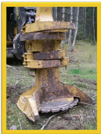
FIGURE 7. A feller-buncher head. The rotating saw blade can create sparks when it strikes a rock.
