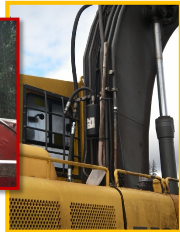
FIGURE 4. Shovel mounted directly to a feller buncher.
